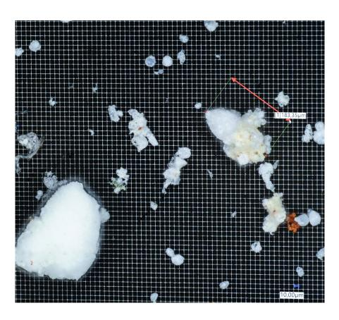
Plastic particles viewed through a 3D microscope at the Institute of Environmental and Process Engineering at RhineMain University of Applied Sciences. The specific dangers posed by microplastics or the even smaller nanoplastics - are currently still the subject of research. It is already clear that particularly small particles can penetrate cells and trigger reactions there. These nanoparticles are found in cosmetics, for example. Photo credit: Arne Dedert/picture alliance via Getty Images
